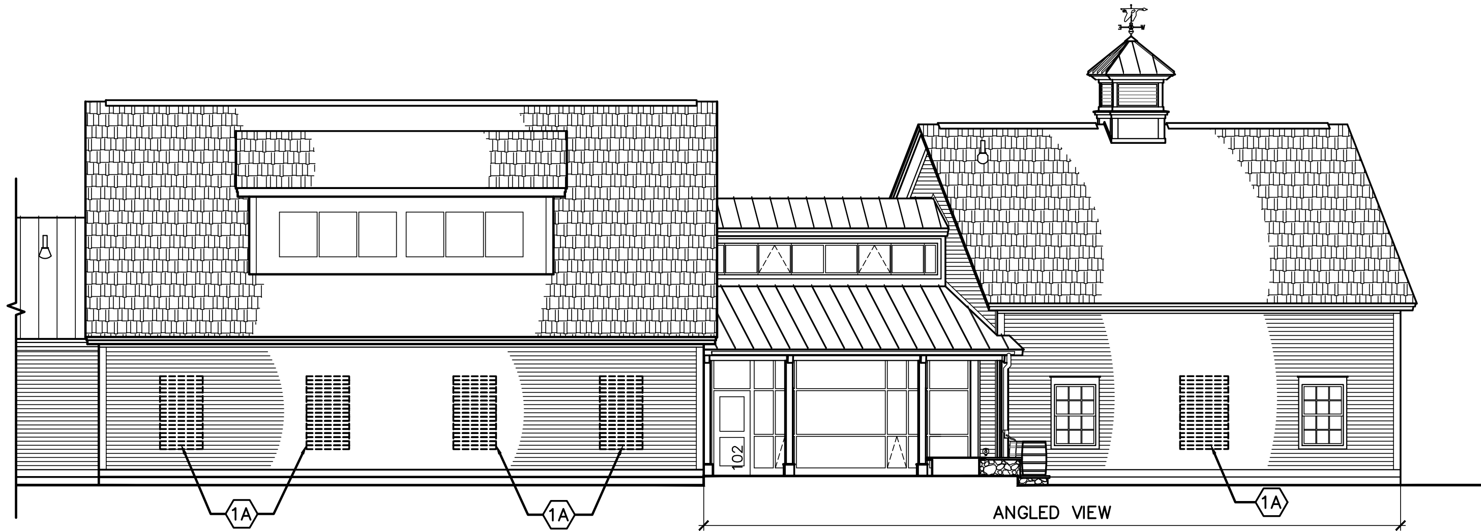
1 NORTH ELEVATION REMOVALS AE201 SCALE: 1/8"=1'-0"
