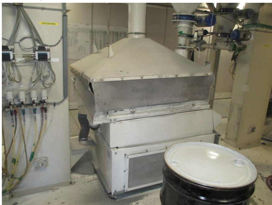
Photo 6: Typical view of the shaker table associated with the blast media recycling process in the ASF.
