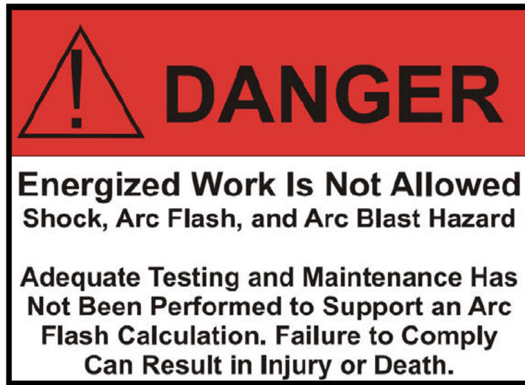
Figure 7-5 Existing Equipment Without Maintenance or Testing
